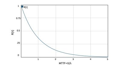
Figure 2: Curve showing the probability that a component is still operational over time
