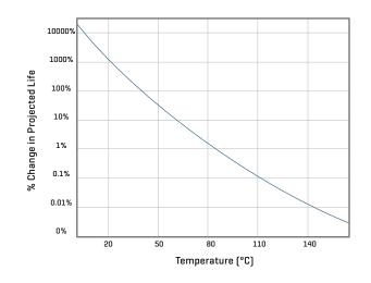
Figure 6: Effect of temperature on a component's projected life. Plot is based on a component rated for 85°C and an activation energy (E<sub>o</sub>) of 1.0
